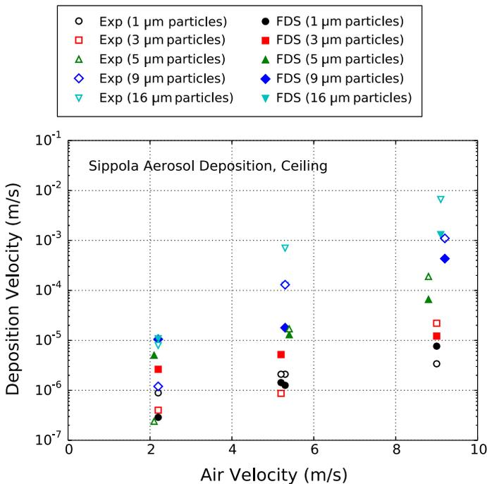
**Figure 5. Measured and predicted ceiling aerosol deposition velocities.**
