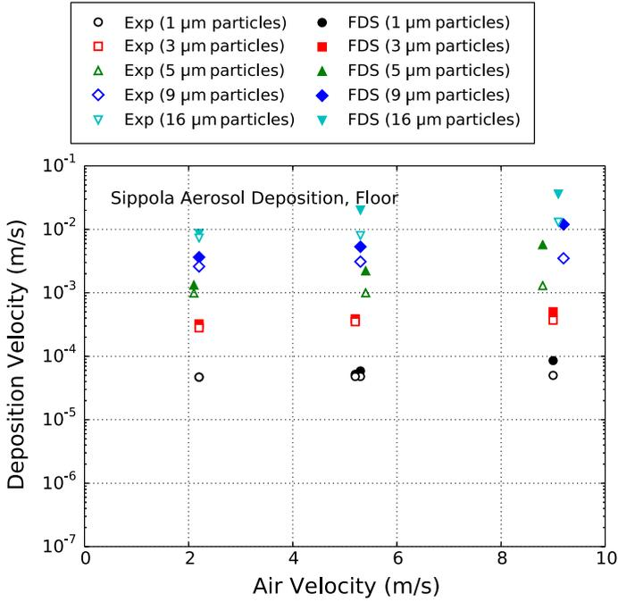
**Figure 7. Measured and predicted floor aerosol deposition velocities.**
