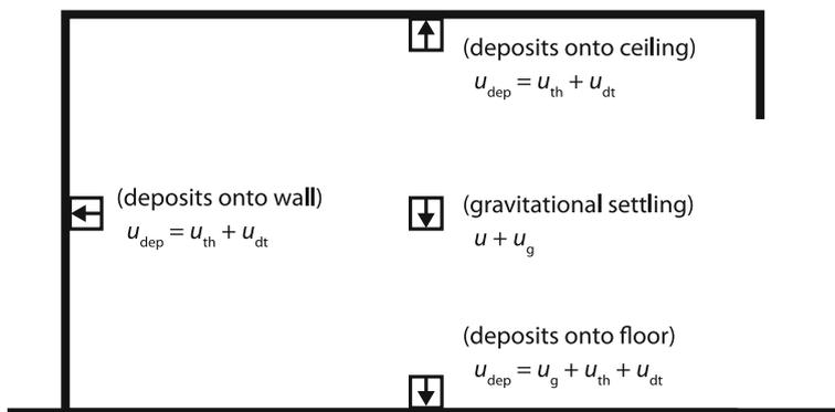
**Figure 3. Soot deposition in a simplified compartment via various mechanisms. Representative computational cells are shown in four different locations: one in the middle of the compartment, and three others near the ceiling, wall, and floor.**
