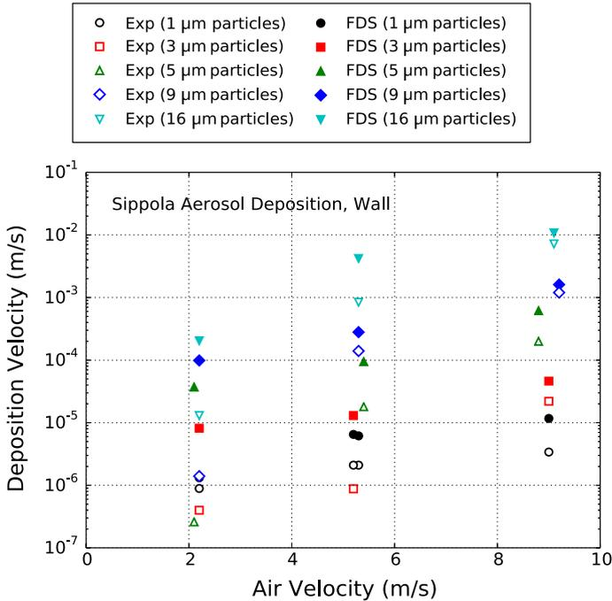
**Figure 6. Measured and predicted wall aerosol deposition velocities.**
