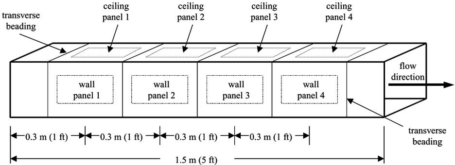
(b) Detailed view of instrumented duct Section 2
