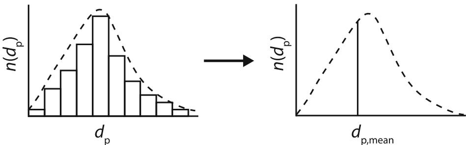
**Figure 2. Detailed particle size distribution (left) represented by mean particle size (right).**
